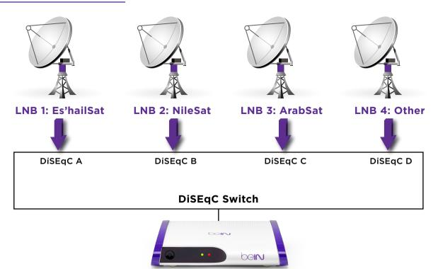
If your configuration does not match the above set-up, change the DiSEqC Port setting to match your set-up.
